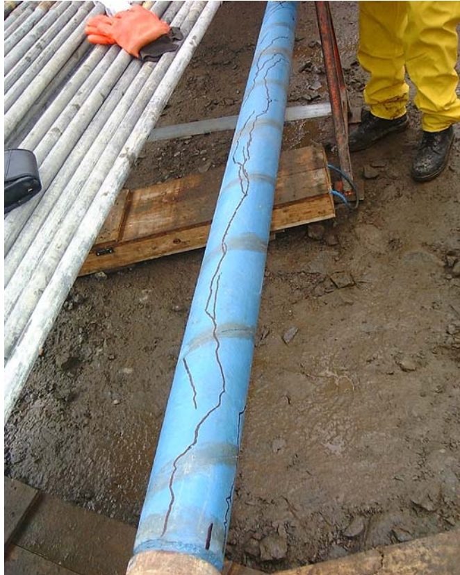
Fig.4: Impression packer with traces of induced fractures
